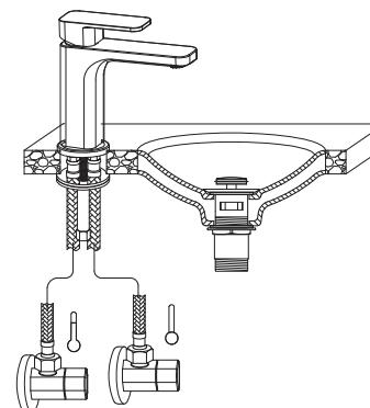
**4.** Fix the two flexible hoses with the hot and cold valve. Open the hot and cold valve to check if there is leakage at the junction.
