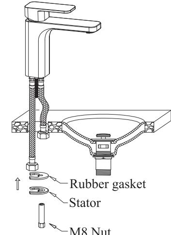
**2.** Take the two flexible hoses individually to go through the hole and then fix the rubber gasket and stator with the M8 screw stem.
