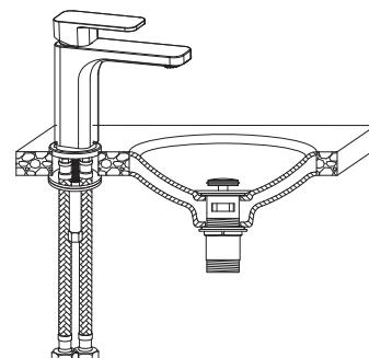
**3.** Adjust the stator, ensure it is at the bottom center of the hole. Fix the hexagon nut while remaining the correct direction of the tap flow. Fasten the hexagon nut until it's firm enough.
