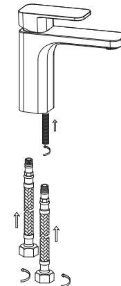
**1.** Fix the M8 screw stem into the M8 screw hole of the mixer. Assemble the two flexible hoses with the tap.
