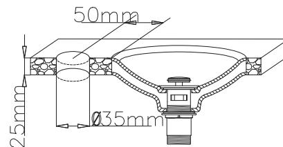
Make a hole with diameter 35mm on the deck 50mm from the edge.
